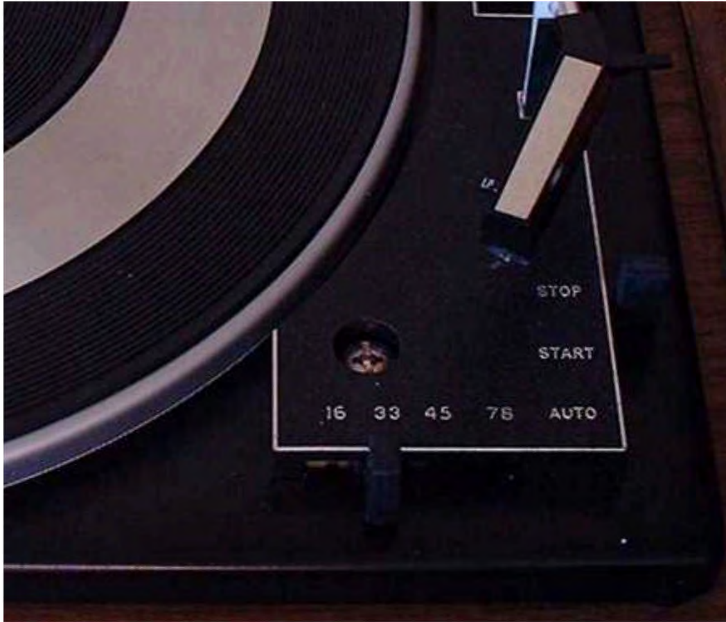
Fig. 8: 1960s turntable with 16-rpm speed setting. Source: 16rpm.com.
