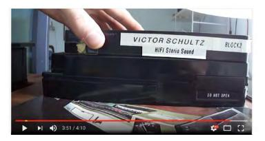
The housing of the cassette is indented on two corners of the same side. This was an ergonomic feature so that the cassette could be gripped when loading and unloading it from the VR-1000 machine. On the top of the cassette, at the same end as the indentions, there is a transparent panel that allows you to see the take-up reel. On the panel are markings that
