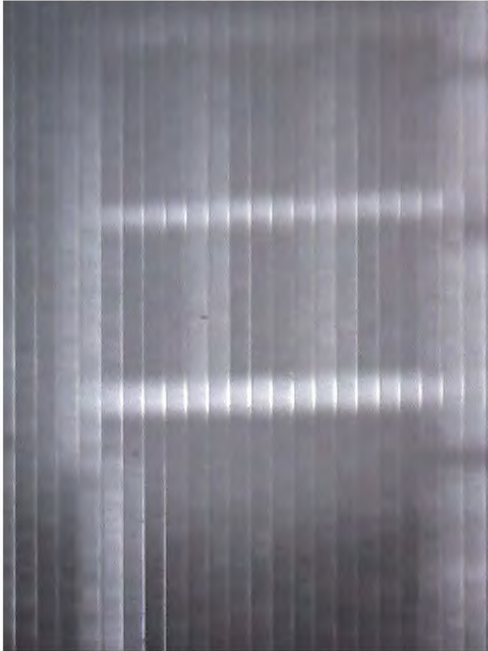
Image 6: Kodacolor's lenticules are visible at 200x magnification. Source: Cumming, Jesse. "Exploring Lenticular Kodacolor" ( http://www.vancouverarchives.ca/2012/12/06/exploring-lenticular-kodacolor/ )
