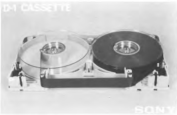
Fig. 7. SMPTE D-1 cassette — internal construction.
