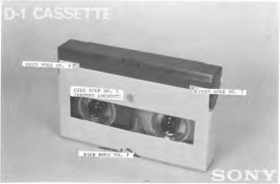
Fig. 5. SMPTE D-1 "S" cassette showing user holes.
