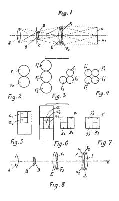
The optical system of Rouxcoloruses a four-color lens to split the images in blue, yellow, red and green. The four separations are recorded on one single frame of a single 35mm film. Each image approximately equals 7.5 x 10.5 mm. The film stock used is the standard black-and-white film which can be processed as one in any lab.
