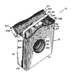
Like many cassettes, Cartrivision had been designed for durability and ease-of use. It contains many features of VHS cassettes, the eventual standard-bearer of consumer home video. Two reels are housed inside the encasing, on which one end is a pivotal closure opened for
